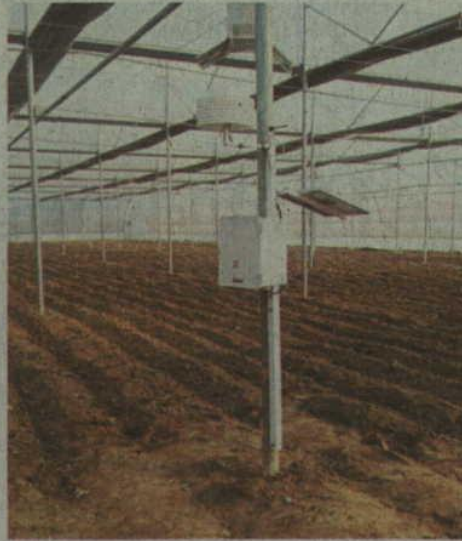
In season An automatic weather station at a potato farm in West Bengal
